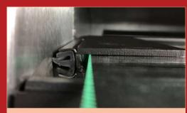
FIXED AGAINST THE FRAME, THE GLASS PANES ARE AIRTIGHT AND PRESERVE THE BAKING QUALITY. THANKS TO THEIR SEALING JOINTS, BOTH HOT AIR AND STEAM STAY INSIDE THE CHAMBER FOR AN EFFICIENT AND ECONOMICAL BAKING.
